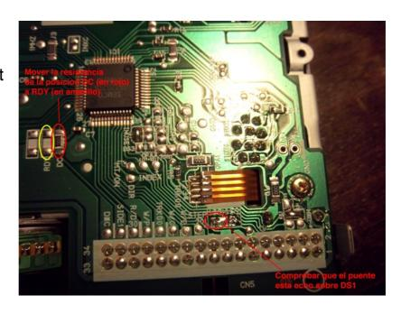
We could also desold the density detector to be able to use any disks without the need of adhesive tape. In this case we need to make sure position C19 is open (no connectivity).
