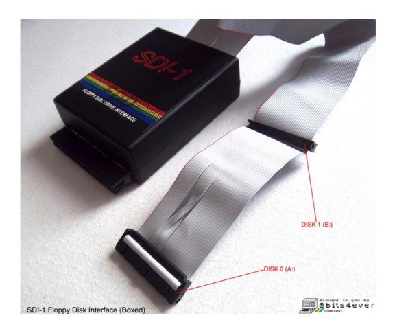
With a special ribbon cable (not included) the SDI-1 will also allow to connect 3" disk drives, like the ones included on the Spectrum +3 for example. This option is very useful if one wants to run software from original 3" disks.
