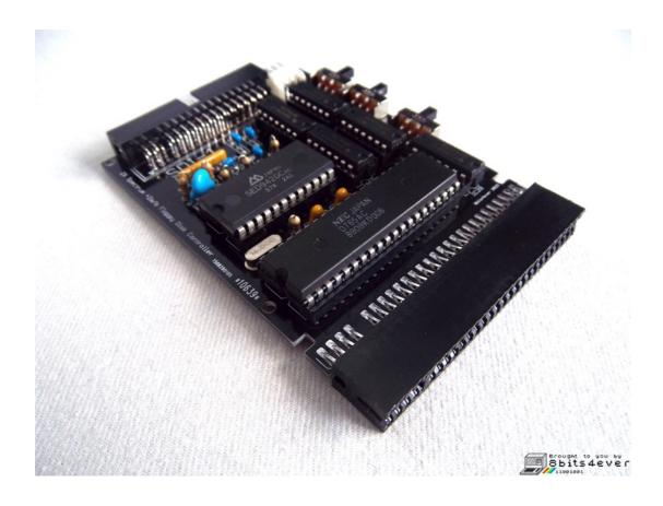
The SDI-1 Disk Interface is specially designed to be used with the Sinclair Spectrum +2a/b computers. It is not compatible with any other models on the Sinclair Spectrum line.
