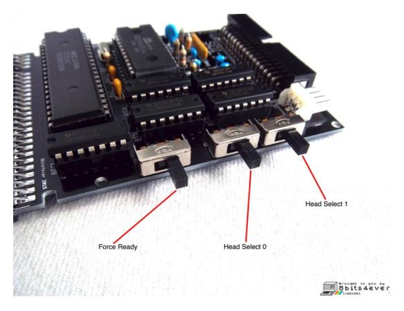
inserted. It this particular situation, if a disk access command is issued, the computer will block until a disk is inserted or the "FORCE READY" switch is put back to "OFF" position.
